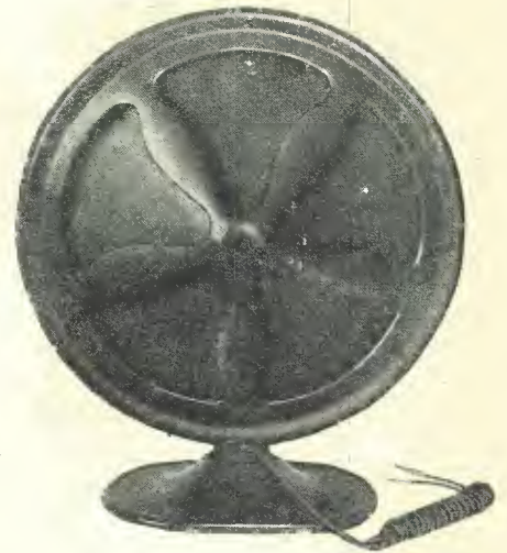
Left: The back of the cone speaker, with the silk cover removed to show the position of the drive-unit on the upright section of the frame. Right: The front of the same speaker. Illustrations courtesy Bondette Mfg. Co.
